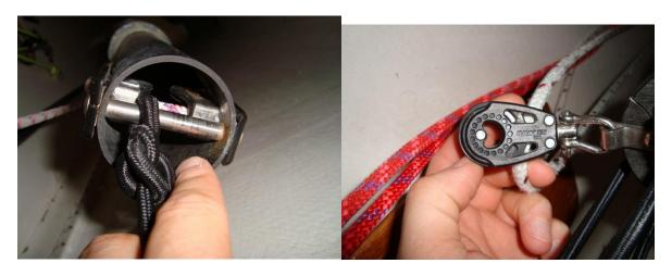
Step 3) move cleat on deck. Depending on your boat, this may require adding a thru deck block as well. We recommend using a double thru deck like a Harken 089. This allows the line to turn the corners thru the deck and run forward without chafing. A single thru deck will not turn the line forward, only down.
