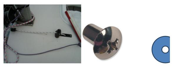
Step 4) re-run the line. This may be easier by removing the outboard end of the pole and sliding the pole into the hull. Getting the line through the two bushings will probably be the most difficult part of the project. You may need a longer tack line than you previously had since both pole out and tack are together. The line should be sufficiently long so if the clew is held by the crew, the tack can stream behind the boat, preventing shrimping.
